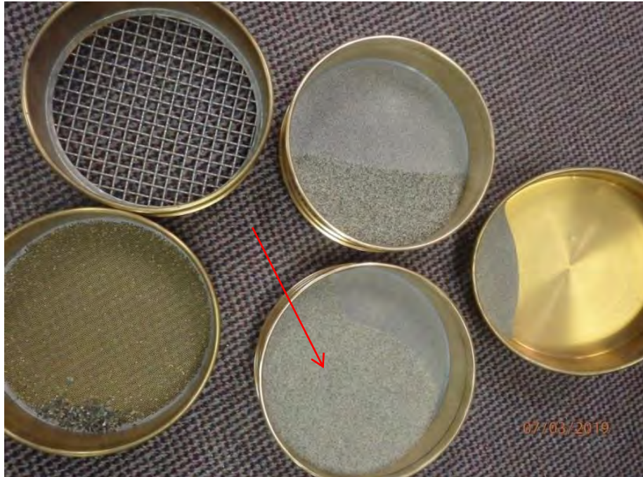
RETAINED FRACTIONS OF SEDIMENT FROM A SAMPLE TAKEN FROM BEACH UNIT 4 (SIDNEY ISLAND). NOTE ABUNDANCE OF SEDIMENT IN THE 0.21 - 0.42 MM FRACTION (HIGHLIGHTED), INDICATING POTENTIAL PSL SPAWNING HABITAT.
