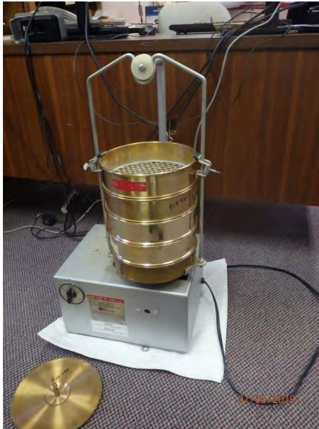
STACK OF SIEVES (9.5 MM, 1.0 MM, 0.42 MM AND 0.21 MM) AND SHAKER MACHINE USED FOR THE GRAIN SIZE ANALYSIS.
